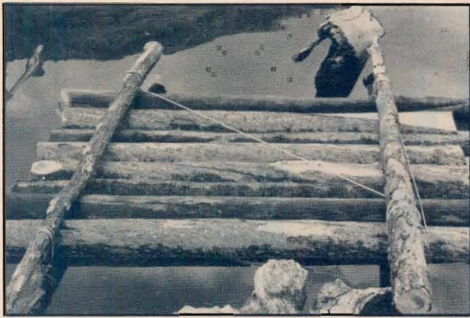
ABOVE — The pressure bar raft can be constructed with a 50-foot rope.
